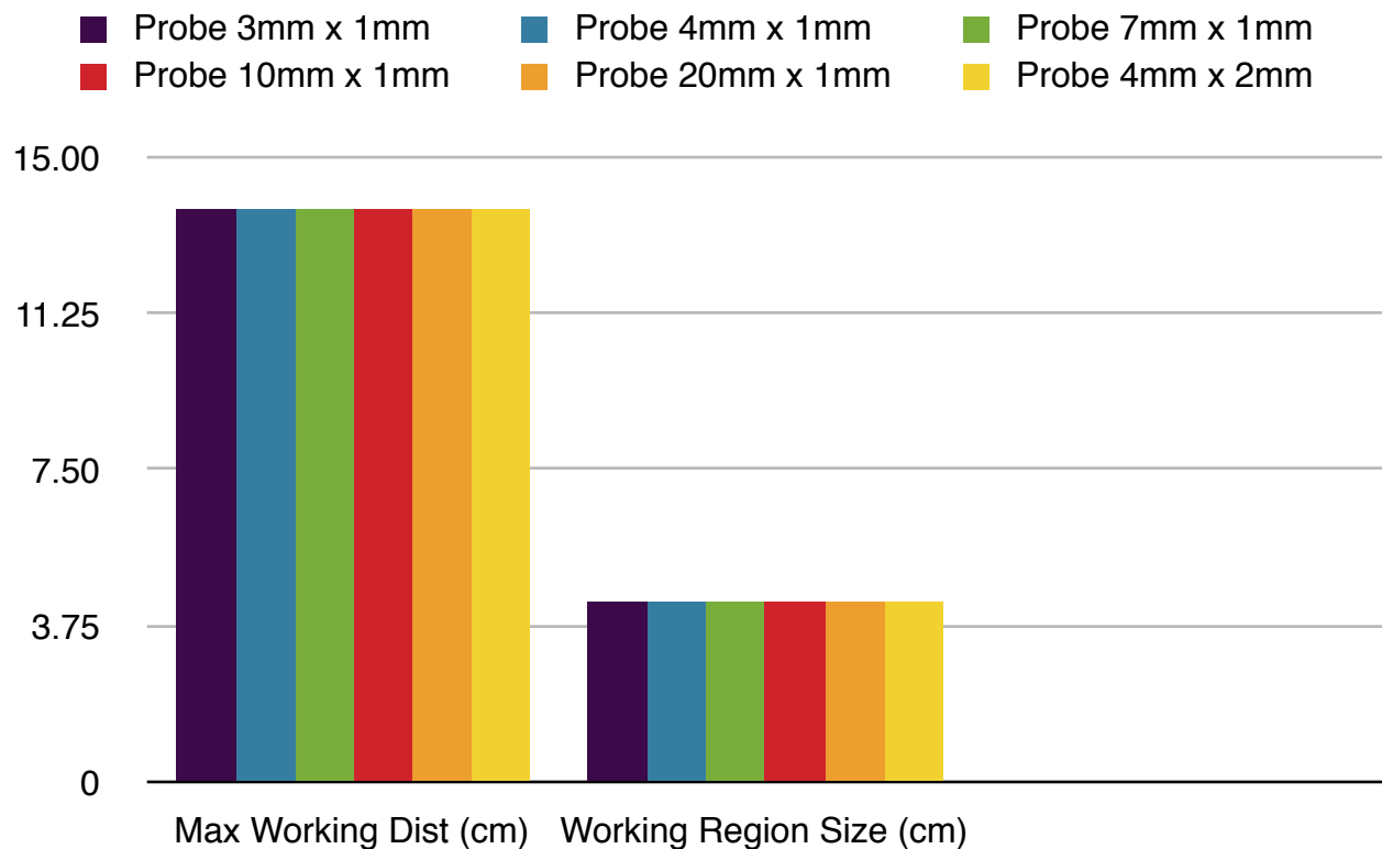
Figure 3: In the on-axis configuration, both the maximum working distance and the operating region size are independent of probe size . This is because the force of gravity acting on the probe, and the magnetic force, are both proportional to the volume of the probe. A physical experiment was conducted to calibrate the simulator. Results indicated that the maximum working distance for a cylindrical 1mmx4mm probe actuated by a cylindrical 37mmx37mm magnet matched the simulation results to within the 0.5cm measurement error of the experimental setup.
